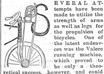
made to utilize the strength of arms as well as legs for the propulsion of bicycles. One of the latest endeavors was the Valere running machine, which proved to be only a theoretical success, however, and could
