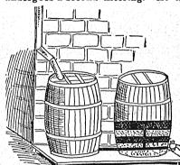
oottom of this cask the water, twice filtered, is drawn off for use. Water from a pump, whether from a well, river or tank, may be as readily filtered in this manner as cainwater.
