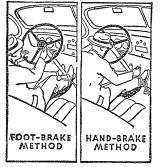
cars from rolling backward, put their engine in low gear and accelerate slowly with the hand throttle, gradually engaging their clutch and releasing the brake at the same time. Other good drivers do exactly the same thing, only they use the hand brake and the foot accelerator. But both groups tell us it doesn't make much difference . . . whichever method we happen to like the
