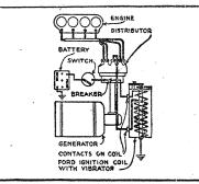
How the Vibrating Coil Is Connected.
