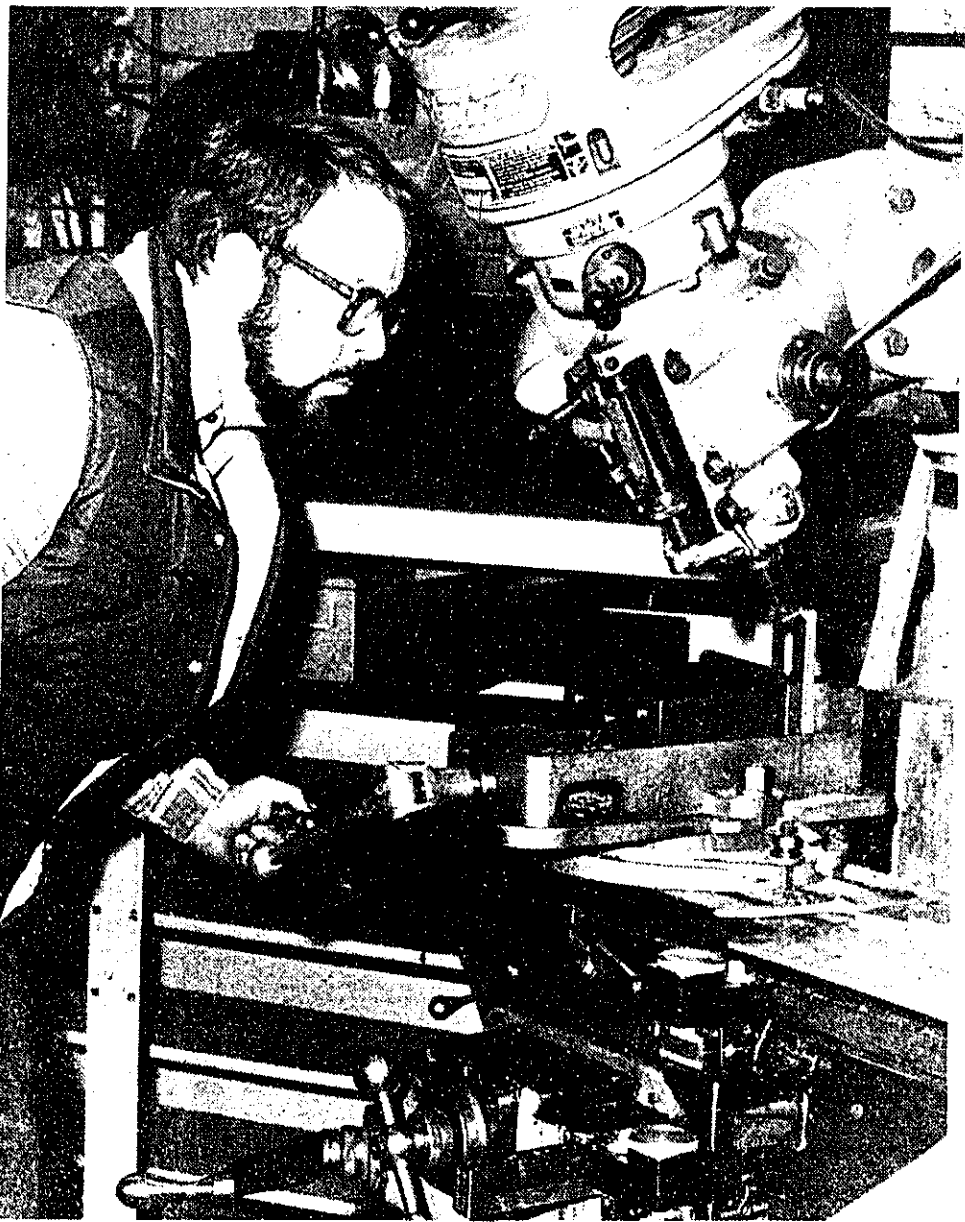
MILLING -- Dave Sturtevant uses a milling machine to bevel an edge on the part.
