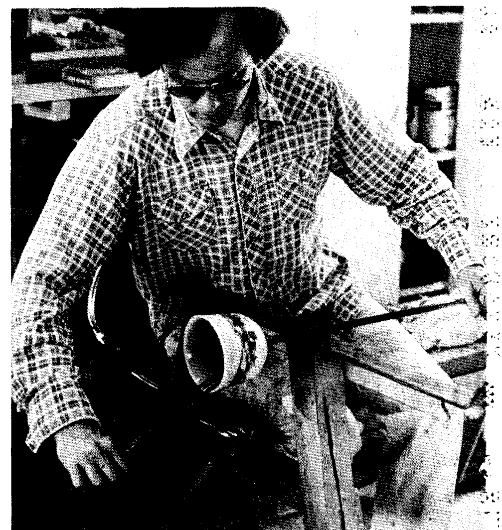
SHAPING -- While the glass is still soft, the opening is shaped. A small opening and shaping makes it a vase; a bigger opening, it's a bowl. Spin the blowpipe enough and it becomes a plate.
