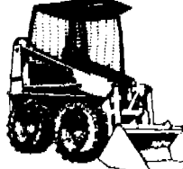
MODEL 1830 Hydrostatic drive 32 hp (23 kW) water cooled engine
