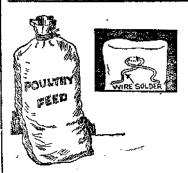
Wire solder holds better, tasts longer than twine when used as fastener on sacks of poultry or stock foods. Stitched through the sacks as shown, solder stays al-
