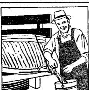
Tank spigots are subjected to heavy wear and tear, being continually bumped by some passing object or broken loose by the weight of heavy water buckets. This may be prevented by welding braces in the manner shown above. Added support will make it possible for spigot to with-
