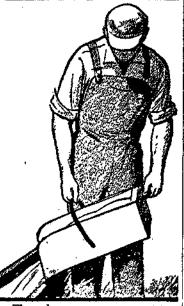
The above scoop may save considerable time for a number of farmers. It can be made from two-foot piece of sheet metal nailed to a wooden square. Bail is off center for easy tipping.
