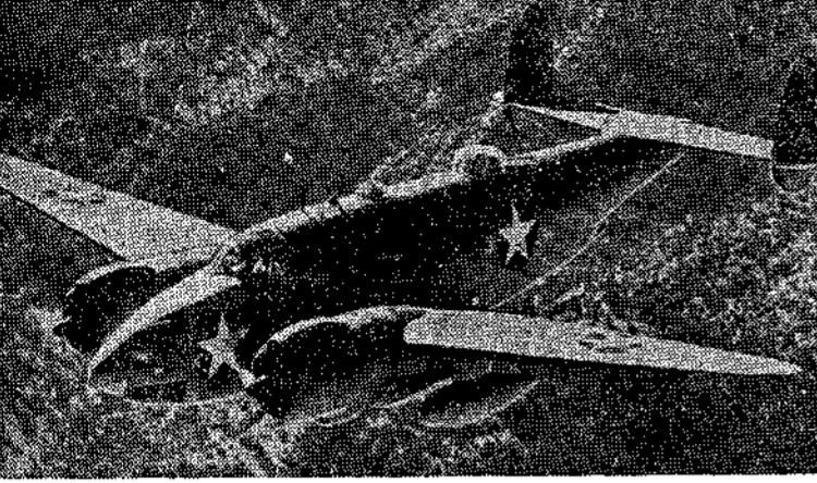
Hailed as the new scourge of the submarine, this mighty new land-based patrol plane, the Vega PV-1, may prove to be the navy's answer to undersea warfare. The PV-1 carries "ash can" depth charges, or torpedoes, and is the first sub-buster in production to fill the navy's need for twin-engine, land-based aircraft with plenty of range and striking power.
