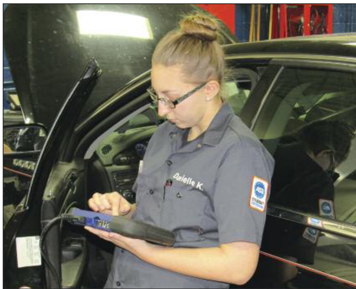
CASS CITY High School senior Danielle Kopah, an automotive technology student at the Tuscola Technology Center in Caro, utilizes a diagnostic tool to "talk" to a car's computer system in order to find out why the vehicle won't start. The patch on her shirt signifies that Kopah has earned the ASE (Automotive Service Excellence) student certification.
