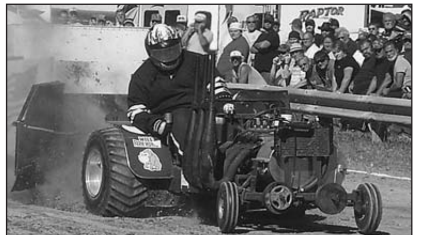
ALYNN HUDSON of Decker has been pulling with M-T Pocket Pullers for 10 years with his tractor, 'Wild Farm Monkey.' He pulls in the 581-800cc Ultra Lite Class. Wild Farm Monkey is unique in its class because the tractor is powered by a snowmobile motor.
