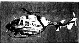
THE FLIGHTCARE helicopter can carry 2 patients along with the flight and medical crew. The craft has a cruising speed of 150 miles per hour and a range of about 250 miles.
