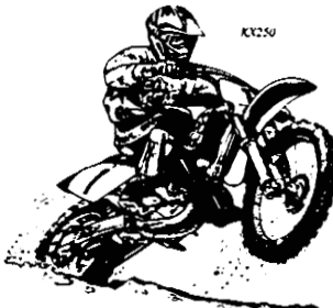
• 2-Stroke, Liquid-Cooled 240cc Engine • Kawasaki Integrated Power-Valve System • New 4-Speed Front Fork • Bottom-Link Uni-Trak® Linkage • High-Tensile-Steel Perimeter Frame
