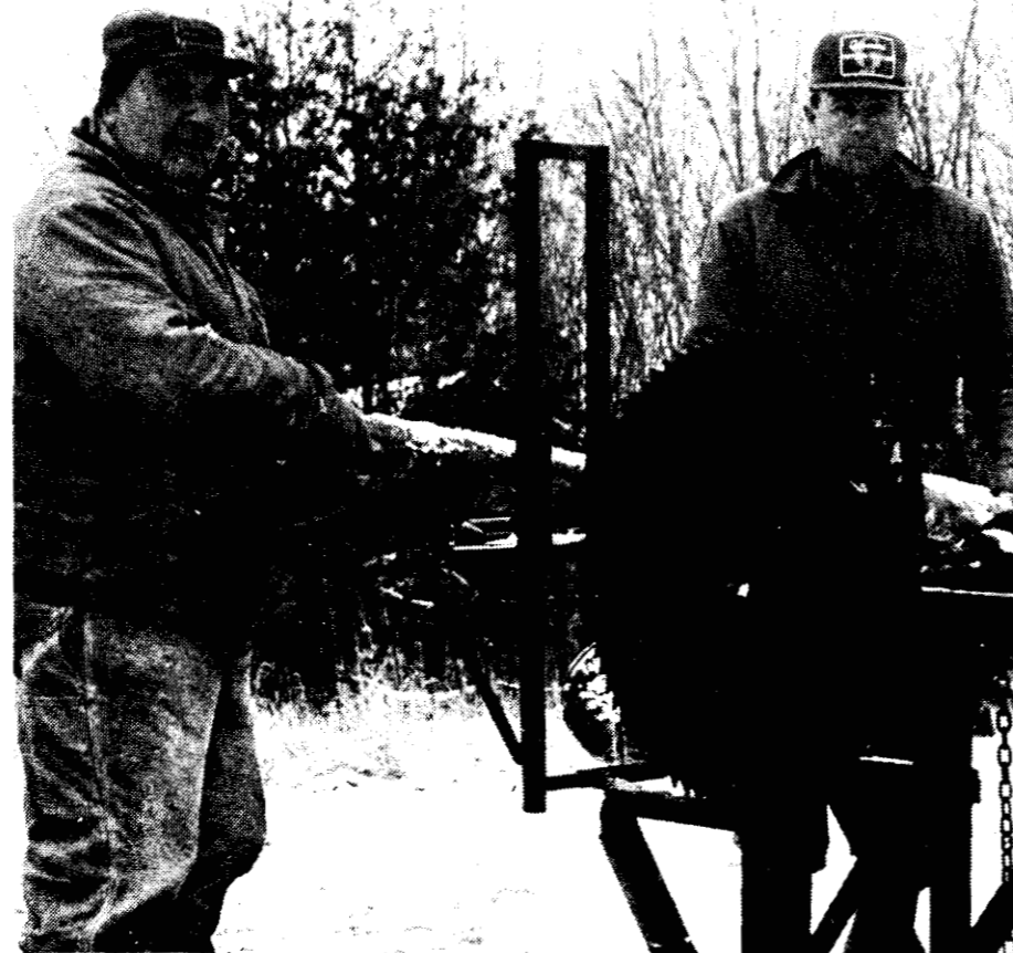
ART (LEFT) AND MARK BATTEL GET set to run a log of popple through their homemade buzz saw, which cuts the long section of wood into fire length portions. The large circular blade is connected, with belts and pulleys, to a farm tractor for power.
