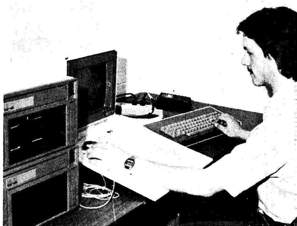
COMPUTER AIDED DESIGN -- William Holdburg, a second year drafting student, designs a part on the computer display screen. When the design is completed, the plotter, shown below, makes the drawing in a couple of minutes.
