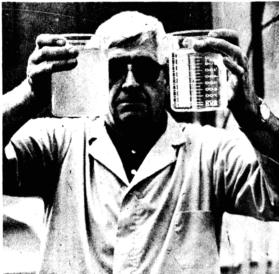
BEFORE AND AFTER -- The beaker on the left held by Nelson Willy contains wastewater as it enters the Cass City sewage treatment plant. The one on the right holds treated effluent, after which it would go into the Cass River.
