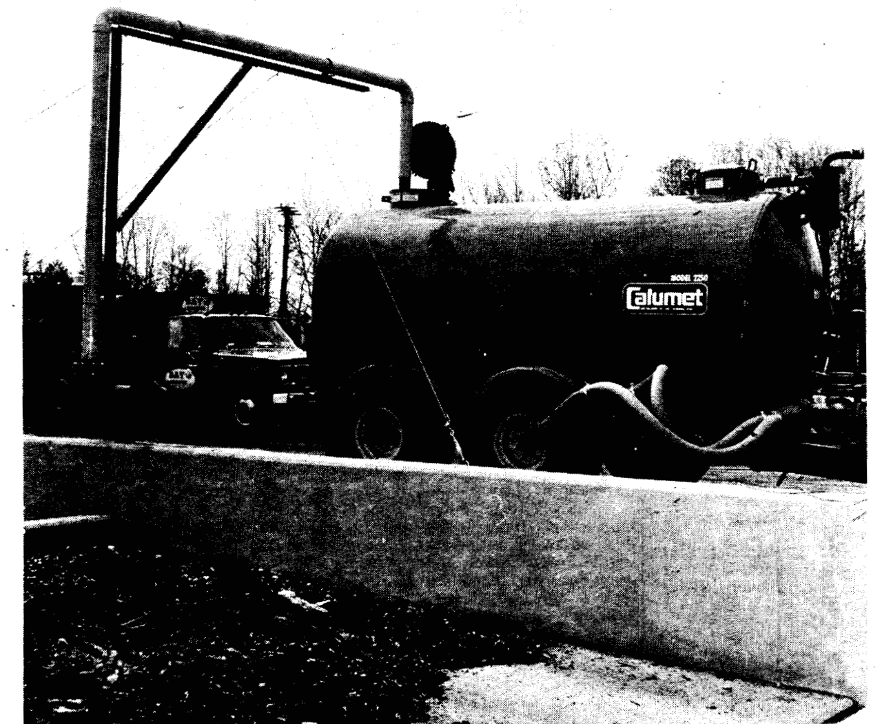
FILL 'ER UP - Cass City's new tractor-towed sludge spreader with its 2,250-gallon tank is being filled with treated sludge at the wastewater treatment plant before being deposited in nearby farm fields.
